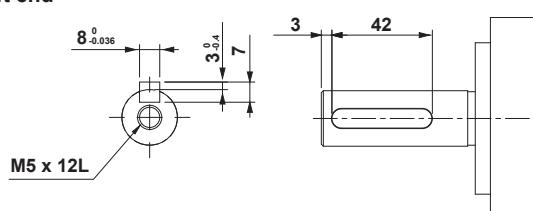
**Type 1500 r/min motors (230 V/400 V, 1.5 kW)**
