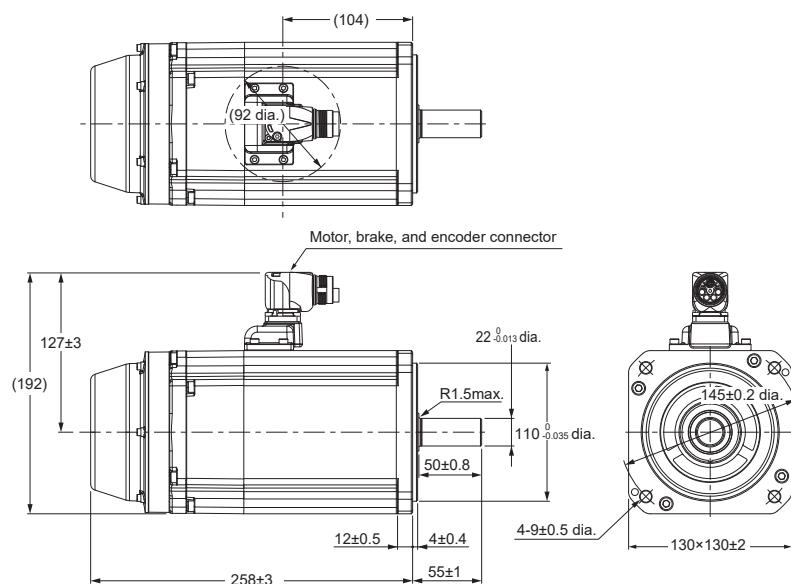
Common dimensions for models with and without brake
