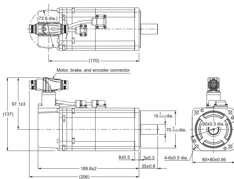
Common dimensions for models with and without brake
