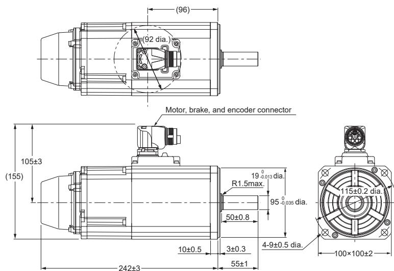
Common dimensions for models with and without brake
