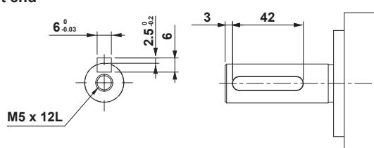
Type 3000 r/min motors (400 V, 3 kW)
