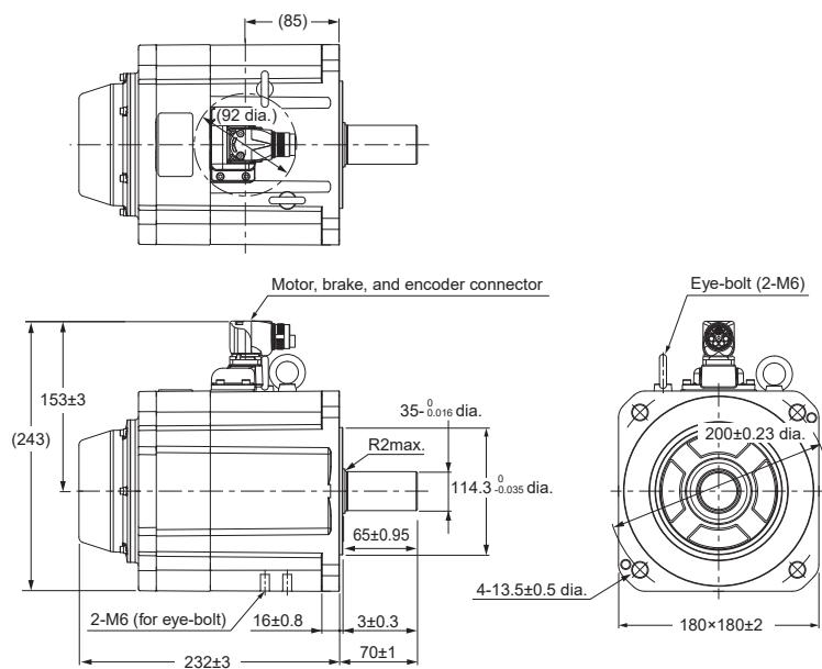
Common dimensions for models with and without brake
