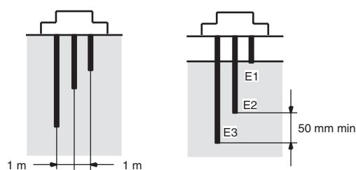
Electrodes are in actual contact with the liquid. Standard electrodes are made of stainless steel and usable in purified water, sea water, sewage, acid (except acetic acid, sulfuric acid, etc.) and alkaline liquids, although they may corrode depending upon the temperature and working conditions.
