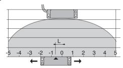
5 mm misalignment tolerance after setting
