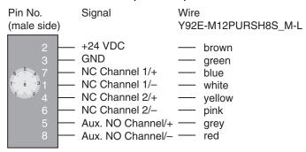
Note: If the auxiliary circuit is not fitted or not used then cut and discard the yellow/green or yellow/pink conductors.
