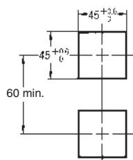
Side-by-side Mounting of N Controllers
