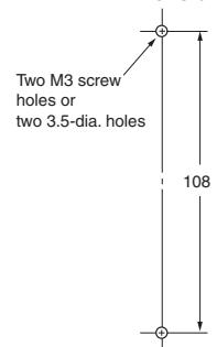
Note: Pull out the hooks to mount the Socket with screws.
