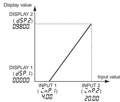
1. Set the K3MA-J input type to the 4 to 20 mA input range.
