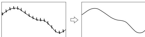
This is useful for ignoring rapid fluctuations, e.g., eliminating spike noise.
