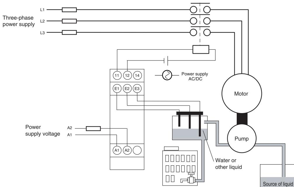
Pump motor protection mechanisms have been omitted.
