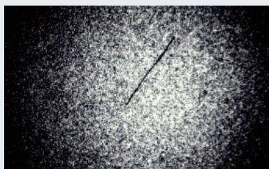
Previous detection image Cannot separate a scratch from noise
