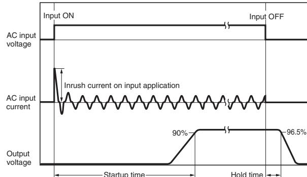
**Note:** Twice the input current or above will flow during the parallel operation or redundant system.
