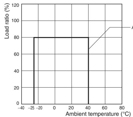
Note: 1. Set the parallel operation switch to the "PARALLEL" side (limit the rated output current to 80%).
