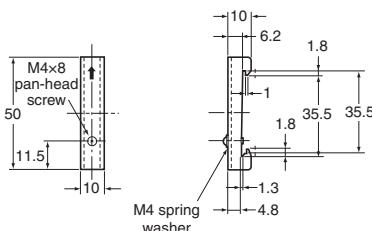
Note: 1. If there is a possibility that the Unit will be subject to vibration or shock, use a steel DIN Rail. Otherwise, metallic filings may result from aluminum abrasion.
