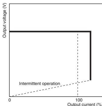
**Note:** 1. Internal parts may occasionally deteriorate or be damaged if a short-circuited or overcurrent state continues during operation. Be sure to check that the  $I_{out} > 100\%$  indicator is not lit or the  $I_{out} > 100\%$  signal output is turned OFF before using.
