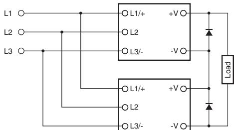
**Note: 1.** If the load is short-circuited, a reverse voltage will be generated inside the Power Supply. If this occurs the product may possibly deteriorate or be damaged. Always connect a diode as shown in the figure. Select diodes with the following ratings.
