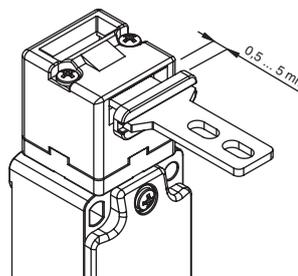
The actuation head of this switch features a wide range of travel. In this way the guard can oscillate along the direction of insertion (4.5 mm) without causing unwanted machine shutdowns. This wide range of travel is available in all actuators in order to ensure maximum device reliability.
