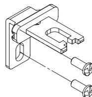
As required by EN ISO 14119, the actuator must be fixed immovably to the guard frame. Pan head safety screws with one-way fitting are available for this purpose. With this screw type, the actuators cannot be removed or tampered by using common tools. See accessories on page 359.
