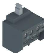
Innovative contact block with 4 contacts, available in various contact configurations for monitoring the actuator or the solenoid (patented). The unit is supplied with captive screws and self-lifting clamping plates. Removable finger protection for eyelet terminal.
