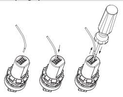
The potentiometer is provided with a three-pole terminal board with PUSH-IN type spring-operated connection. This technology allows a very handy quick wiring procedure. The wire is simply inserted into the appropriate hole, without the need for any auxiliary tooling, through the use of rigid or flexible wires with crimped wire-end sleeve. Release is obtained by pressing the appropriate wire-releasing button.
