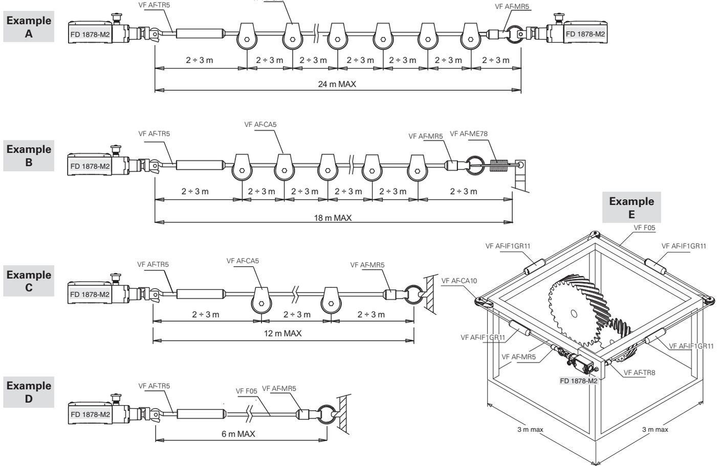
Application examples and max. rope length for switches with transversal head
