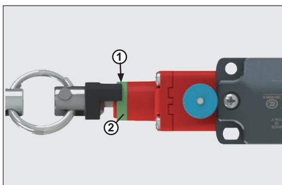
Tighten the rope connected to the switch, until the end of the indicator (1) reaches about the middle of the green ring (2).
