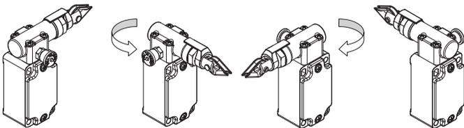
For all switches, the head can be adjusted in 90° steps after removing the four fastening screws.
