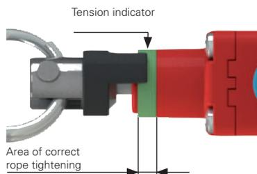
All switches are provided with a green ring that shows the area of the correct tightening of the rope. The installer has only to tighten the rope until the black indicator will be in the middle of the green area. With this setting, the switch can be reset by pulling the blue knob to close the electrical safety
