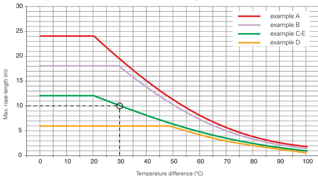
The max. recommended spans are indicated in the diagram as a function of the temperature fluctuations (temperature differences) to which the switch may be exposed at the point of use. For instance, with installation of type C and a temperature difference of 30°C, the max. recommended rope length is 10 metres.
