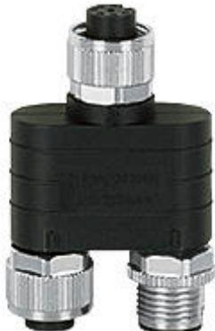
Plug-in connector, Y-adapter, IP67, M12 male connector (X1, evaluationdevice), 8-pin, A-coded on M12 female connector (X2, sensor/ next plug-in connector), 8-pin, A-coded and M12 female connector (X3,sensor), 8-pin, A-coded, incorrect insertion of the connections electricallyexcluded by internal wiring, to connect PSENcode, to directly connect PSENslock on the sensor.
