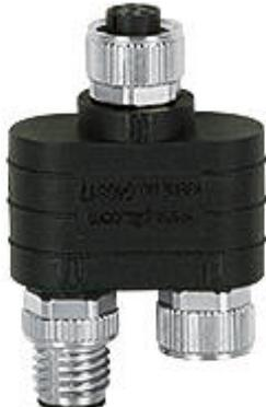
Plug-in connector, Y-adapter, IP67, M8 male connector (X1, evaluationdevice), 8-pin, A-coded on M8 female connector (X2, sensor/next plug-in connector), 8-pin, A-coded and M8 female connector (X3, sensor), 8-pin, A-coded, incorrect insertion of the connections electrically excluded by internal wiring, to connect PSENcode, to directly connect PSENslock on the sensor.
