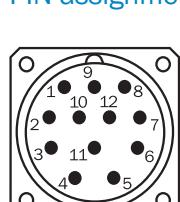
view of M23 male device connector on encoder
