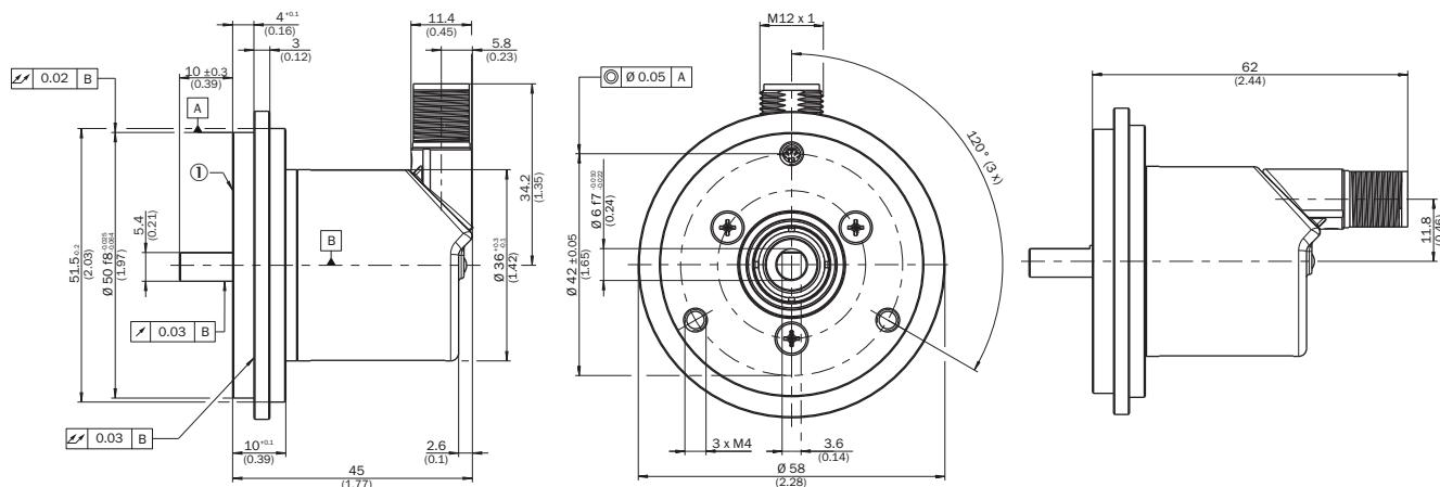
order example for 6 mm shaft diameter: AHx36x-S3xx0xxxx + BEF-FA-020-050 (adapter is not pre-assembled)
