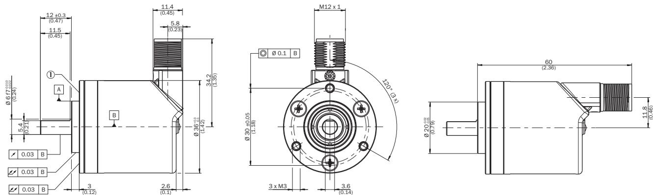
order example for 6 mm shaft diameter: AHx36x-S3xx0xxxx + BEF-FA-020-036-002 (adapter is not pre-assembled)
