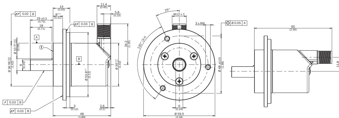
order example for 10 mm shaft diameter: AHx36x-SCxx0xxxx + BEF-FA-020-036 (adapter is not pre-assembled)
