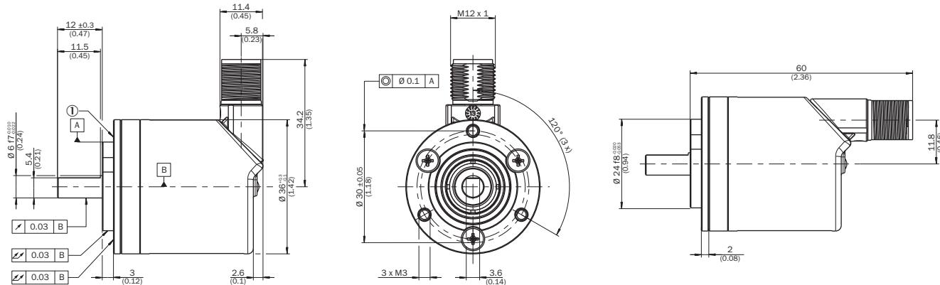
order example for 6 mm shaft diameter: AHx36x-S3xx0xxxx + BEF-FA-020-024 (adapter is not pre-assembled)
