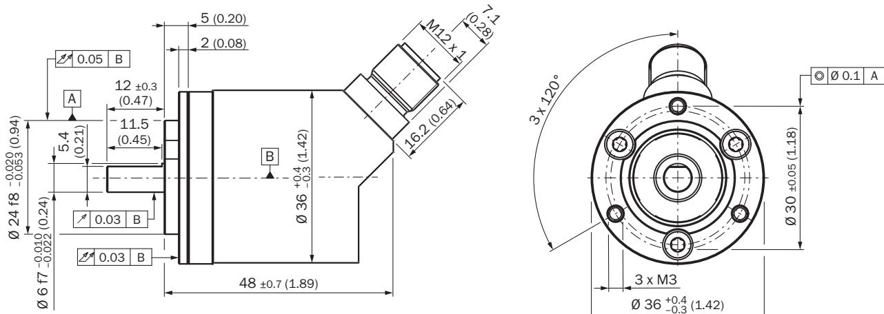
order example for 6 mm shaft diameter: AHx36I-S3xx0xxxx + BEF-FA-020-024-I (adapter is not pre-assembled)
