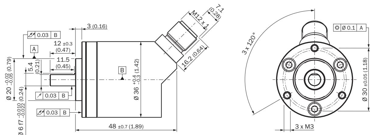
order example for 6 mm shaft diameter: AHx36I-S3xx0xxxx + BEF-FA-020-036-2-I (adapter is not pre-assembled)
