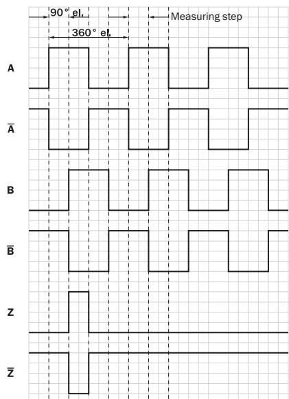
CW with view on the encoder shaft , compare dimensional drawing.
