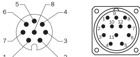
view of M12 male device connector on cable / housing
