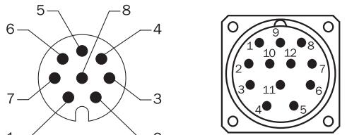
view of M12 male device connector on cable / housing
