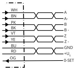
Diagrams Signal Outputs with Counter Clock-wise Counting Direction Option Selected (B leads A for clock-wise rotation). Complement signals AN, BN and ZN are not shown.
