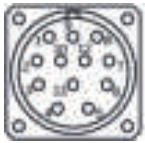
View of the connector M23 fitted to the encoder body
