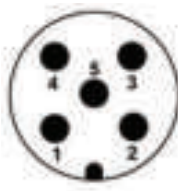
View to the connector M12 fitted to the encoder body
