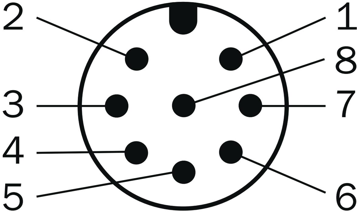
Connector M12, 8-pin, A-coded
