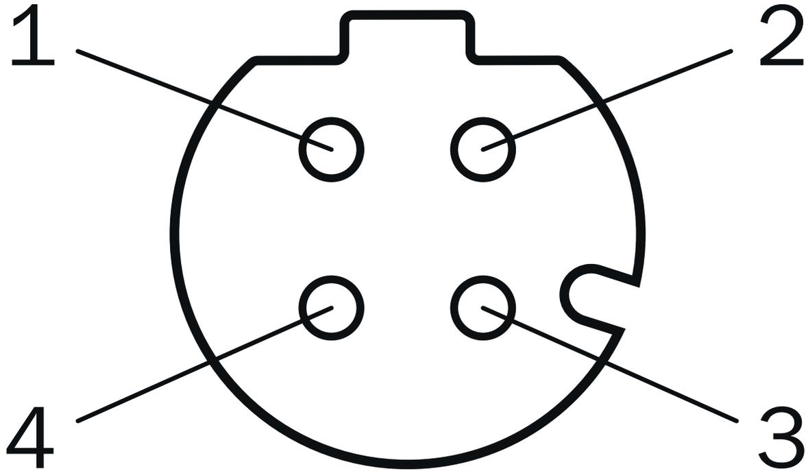
M12 female connector, 4-pin, D-coded
