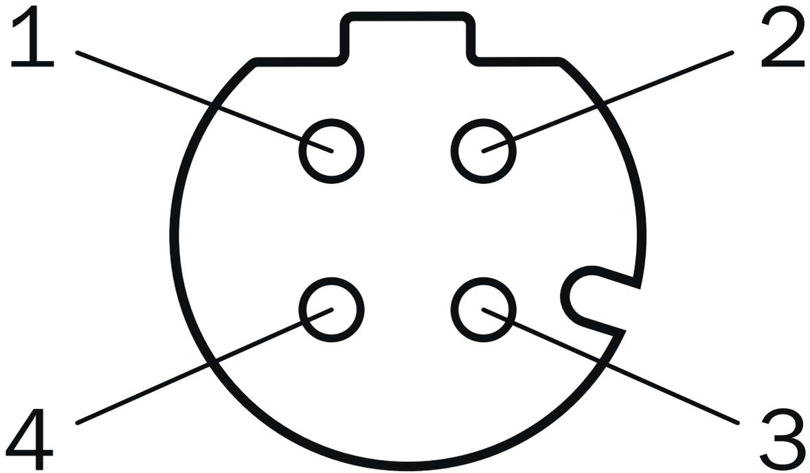
M12 female connector, 4-pin, D-coded
