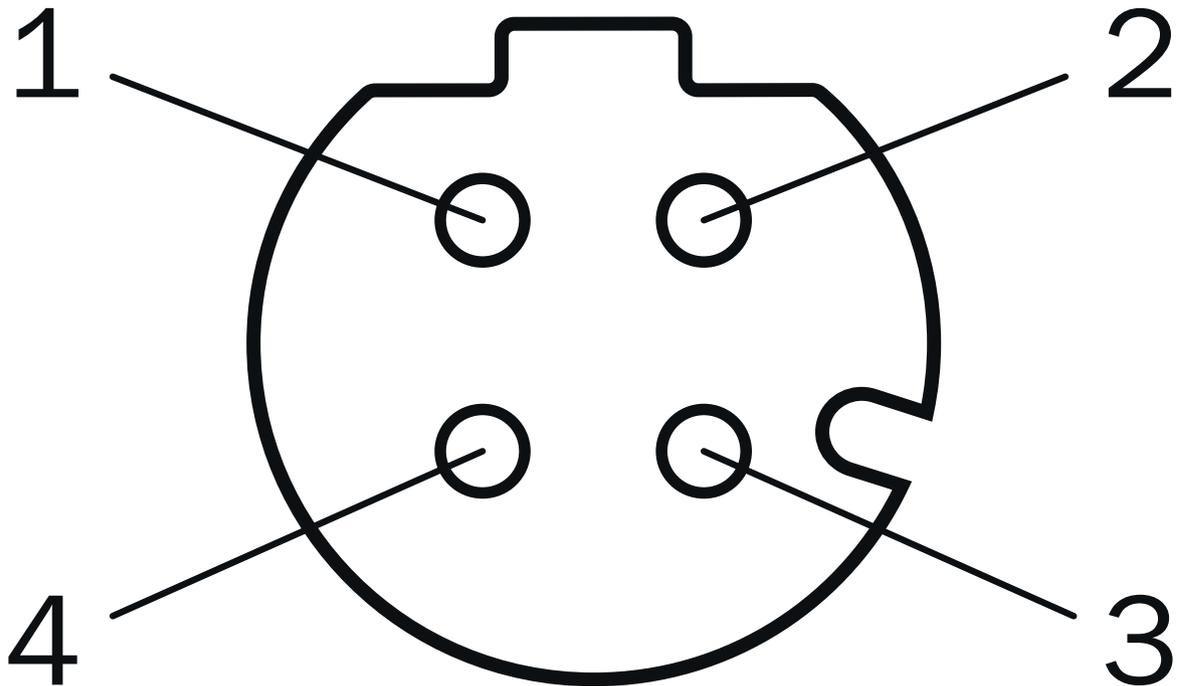
M12 female connector, 4-pin, D-coded
