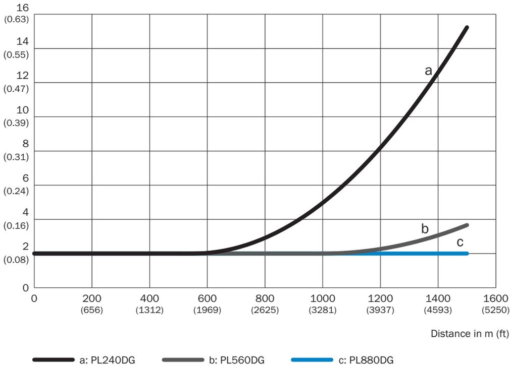
Repeatability DL1000 for various reflector types, with 16 ms measurement cycle time
