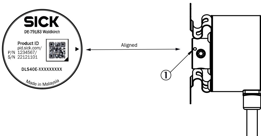
You can see the position with the mark on the rear side of the encoder
