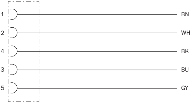
Contact assignment of the M12 female connector
