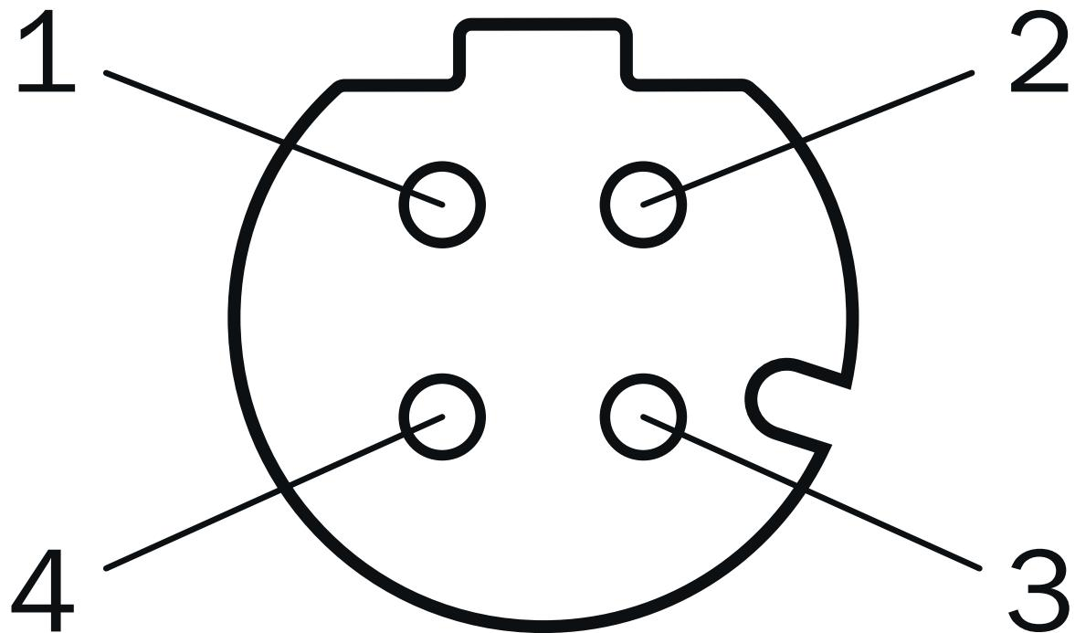
M12 female connector, 4-pin, D-coded
