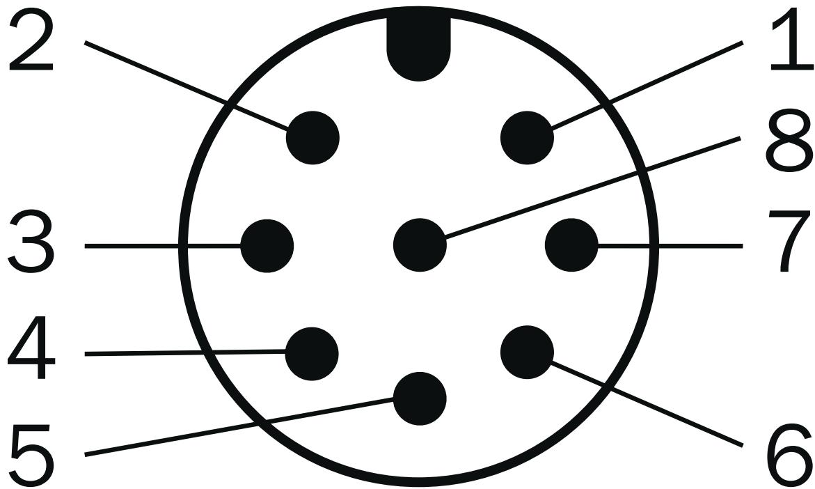
Connector M12, 8-pin, A-coded
