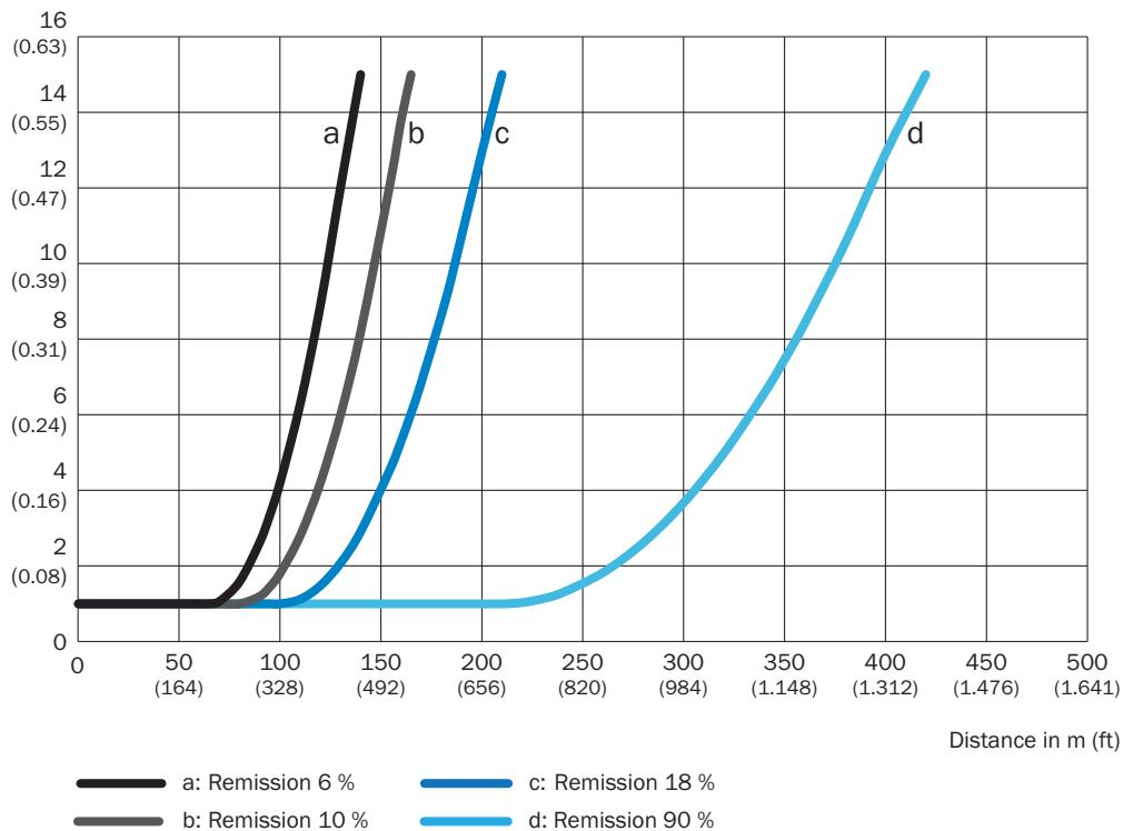
Repeatability DT1000, with 128 ms measurement cycle time
