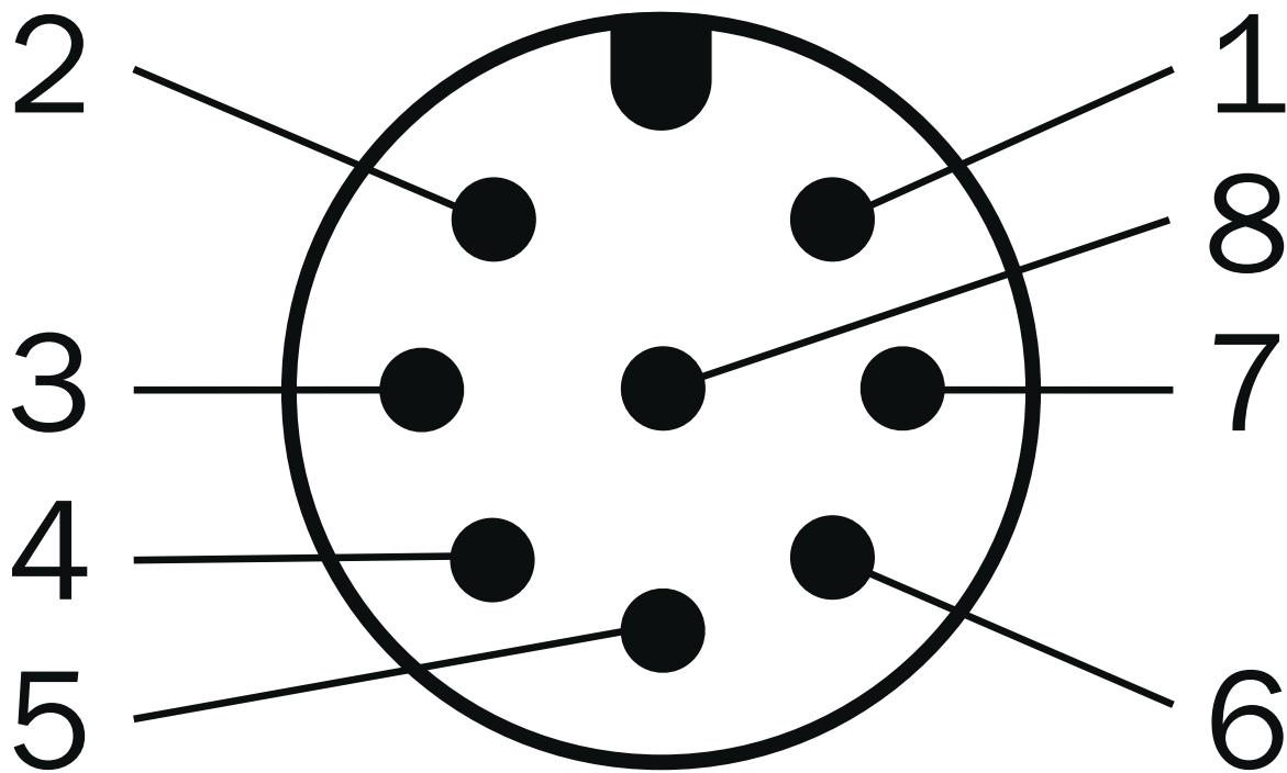
Connector M12, 8-pin, A-coded
