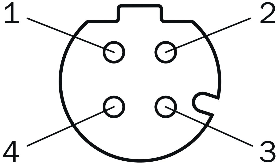
M12 female connector, 4-pin, D-coded
