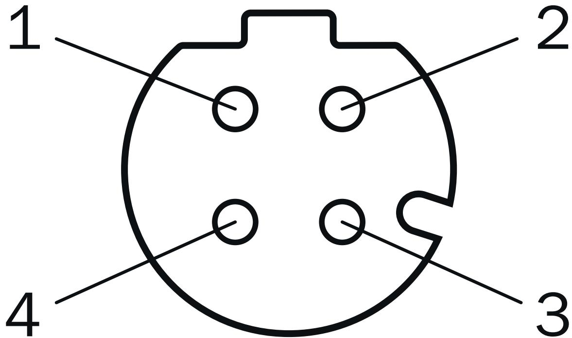
M12 female connector, 4-pin, D-coded
