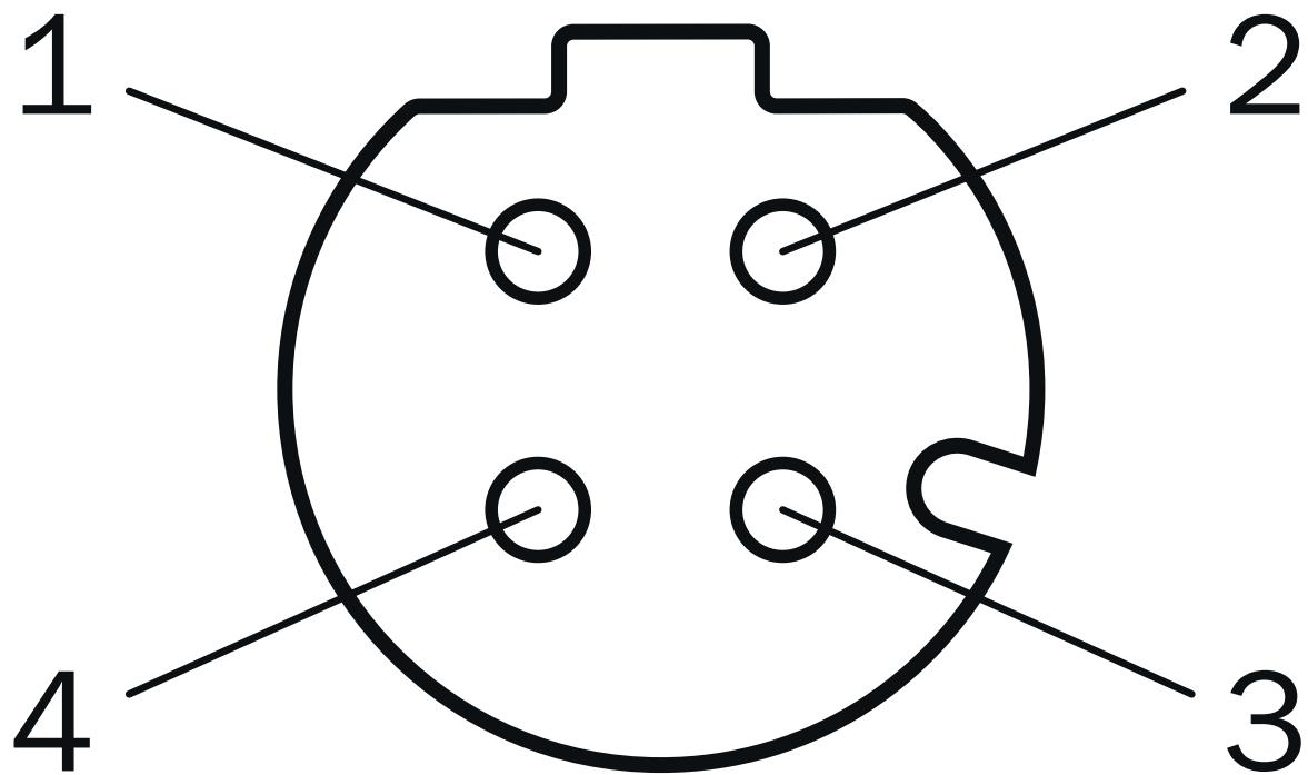
M12 female connector, 4-pin, D-coded
