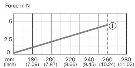
① maximum contact force when the counterweight is positioned at the end of the rod (260 mm)
