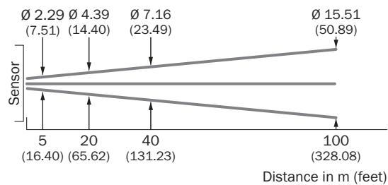
Sensing range diagram GS6-D4311S69, GE6-P4211S69; GS6-D4312S71, GE6-P4212S71
