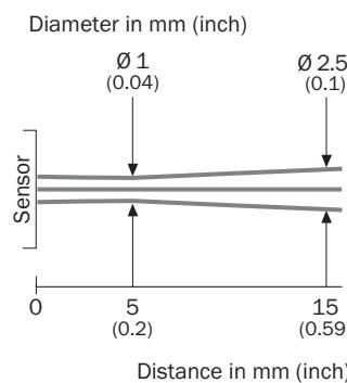
Sensing range diagram GTB2 Flat, 15 mm
