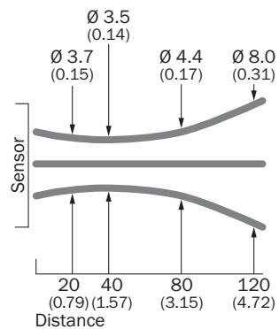
Sensing range diagram GTB2S, 120 mm
