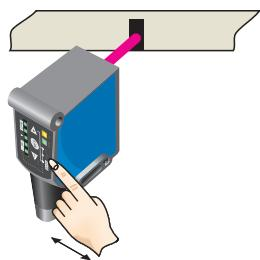
When setting the contrasts to be detected, the first LED (green) flashes in the bar graph. Press set button.
