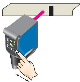
When setting the contrasts to be detected, the second LED (green) flashes in the bar graph. Press set button. The Quality of Teach is displayed.
