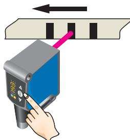
Press the Set pushbutton to end the teach-in process.
