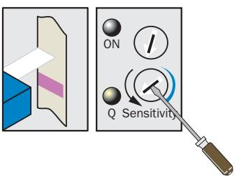
If yellow LED illuminates, turn "Sensitivity" rotary switch counter-clockwise until the yellow LED just goes out.
