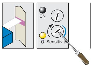
Turn "Sensitivity" rotary switch clockwise until yellow LED illuminates.
