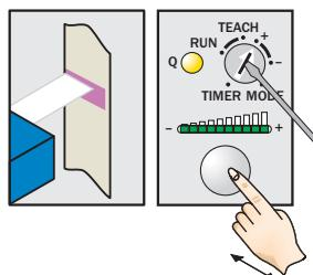
Turn rotary switch to "+" position and press and hold teach-in button until yellow light goes out (more green LEDs illuminate on the bar display).
