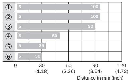
Max. sensing range  $S_n$ , flush or non-flush installation,
