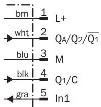
**PIN assignment Connector M12, 5-pin, A-coded**
