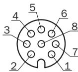
female connector M12, 8-pin, A-coded
