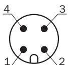
Connector M12, 4-pin, A-coded
