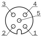
female connector M12, 5-pin, D-coded
