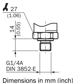
Dimensional drawing Housing with circular connector M12 x 1, IP67
