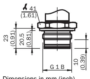
Dimensional drawing Housing with L-connector (DIN EN 175301-803 A)
