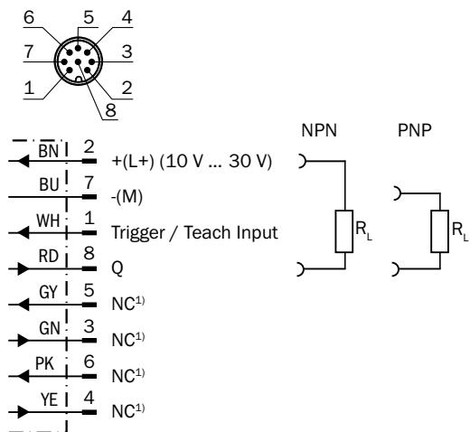
① Not connected. Leave open, do not wire to ground.
