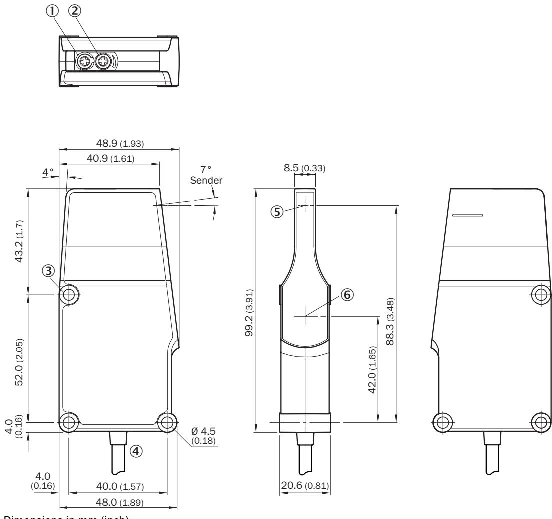
⑥ Center of optical axis, receiver
